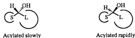
Figure 1. Simple model for predicting which substrates will be resolved effectively via biocatalytic acylations mediated by lipase from Pseudomonas sp. , and the sense of the enantioselection.
